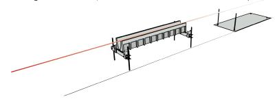
Once the first channel has been replaced, DO NOT lock the adjustable side of the clamp with the wedge yet. This allows some movement of the channel when placing the next channel in line. Do not place the channel all the way to the fixed side of the clamp where it will sit in the locked position. This allows for easier installation of channels.
