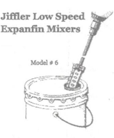
Use key to lower vane: Let shaft stick below hub and tighten screw on flat
