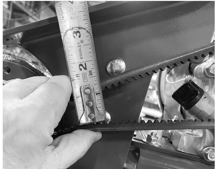
6. Correct belt tension can be checked by using moderate pressure to squeeze both sides of belt. Approximately 1" of movement is correct tension. Loosen engine mounting plate and adjust to correct belt tension. Retighten.
