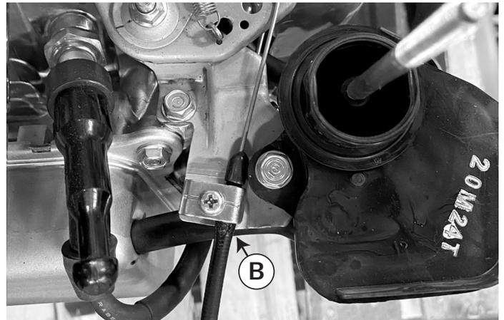
4. The throttle cable/lever comes connected to the handle (A) and carburetor (B). Move throttle lever and watch movement on the carburetor to insure correct operation.
