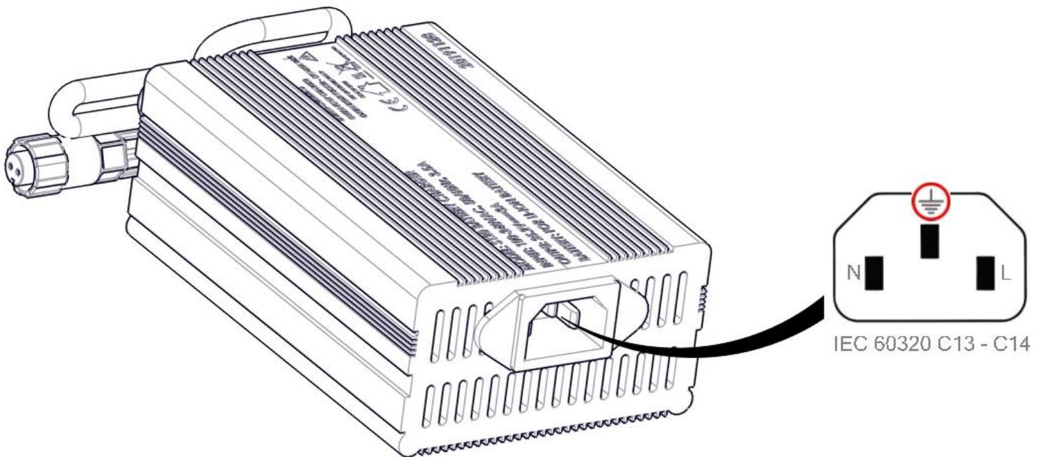
**IF YOU HAVE A PLUG TYPE OTHER THAN (A), YOU CAN USE A IEC 60320 CONNECTOR WITH YOUR COUNTRY PLUG IN THE CHARGER AS LONG AS IT IS RATED AT 250VAC AND 10A.**
