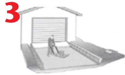
3 Position PointDrain on a 4" thick concrete slurry bed and ensure it is level.
