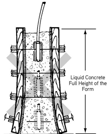
15. Do not exceed the recommended rate of placement and do not continue to place concrete while the concrete in the bottom of the form is still in a liquid state. A form failure may result.
