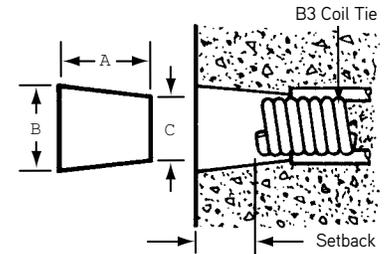
**Warning:** Cones are to be used for spreader action only and are not designed for scaffold bracket or other accessory loads.
