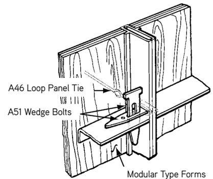
When erecting modular type forms, the A46 ties are placed in the slots between the form panels. An A51 Wedge Bolt is placed through the adjoining form and into the loop of each tie. A second Wedge Bolt is then placed through the slot of the first Wedge Bolt to secure the tie and form together.
