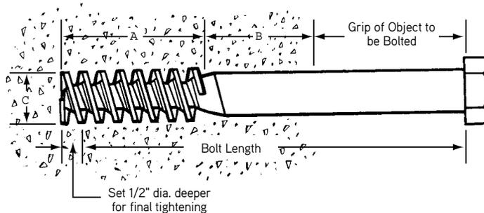
**Assembled Bolt and Anchor**
