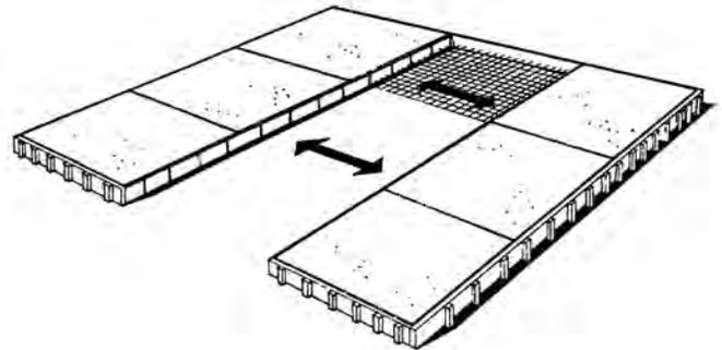
Supports For Rebar and Wire Mesh
