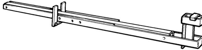
Dayton Superior A90 Scaffold Bracket Jack meets state building codes and OSHA minimum requirements and supports scaffolding on nearly any type of formwork. By changing the position of the pins in the vertical and horizontal members the bracket can be quickly adjusted to fit 2x4, 2x6 or 2x8 wales or positioned flush against a wall.
