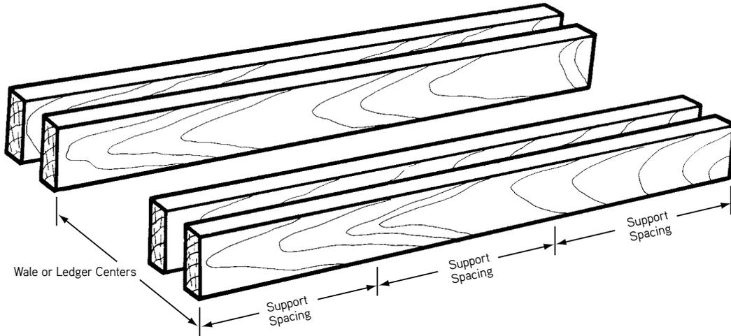
Safe Spacing of Supports for Double Ledgers or Wales Continuous Over Four or More Supports
