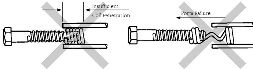
places the entire bolt load on a smaller portion of the coil welds. The increased loading can cause the coil welds to fail and result in form failure.
