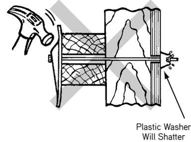
Do not attempt to draw-up warped wales with the wedge. Do not over tighten the wedge in any manner. Over tightening will cause metal spreader washers to bend out of shape or will break plastic cones resulting in incorrect wall thickness.
