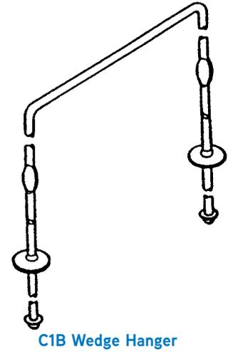
single or double ledgers. This secures the beam bottom against the spreader washers to provide a rigid form and correct depth of fireproofing. C1C Wedge Hangers (without spreader washers) are recommended for use only with soffit spacers.
