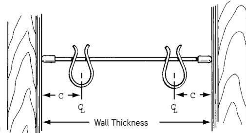
D21 Rebar Clip and Form Spreader
