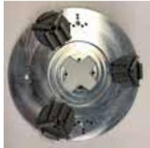
300307 on 200179 tool plate (on Left side with 4 and right side with 3)
