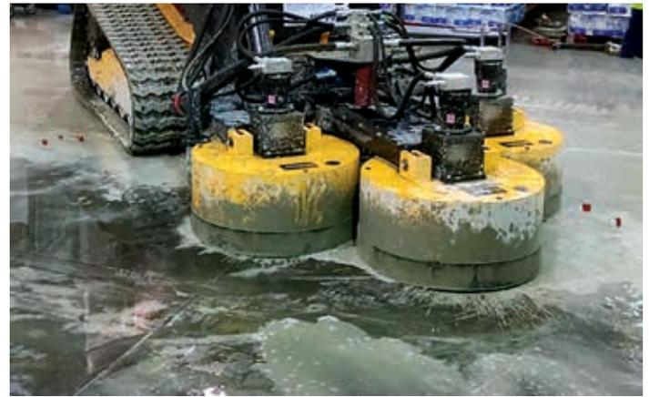
The plates for bolt-on tooling (plate p/n-200179) on the LX30 PRO and Stone Extreme have options for either 3 or 4 bolt-on segments. The hole patterns also include an option for bolt-on traps for even more options. The pin needs to be unthreaded from the universal segments and qty-3 M6 screws per segment must be used to bolt them in place.
