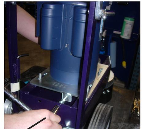
Tighten the belt tensioning bolt until the belts are properly tensioned.
