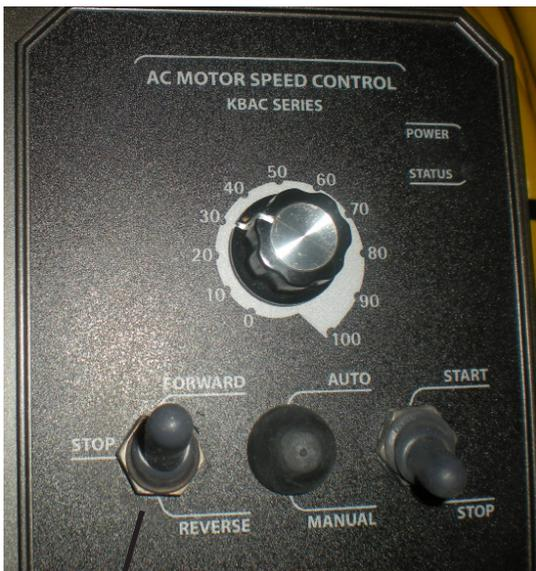
On variable Speed models, be certain the proper rotation for the PCD is made via the FWD/REV switch.
