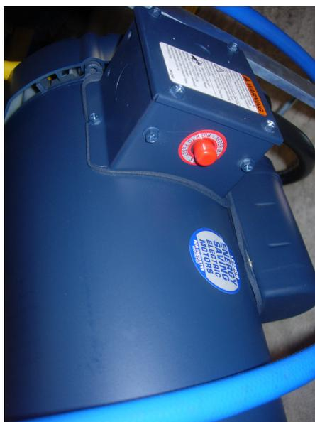
The thermal overload on the motor is located under the motor conduit box (see picture to the left for Leeson and below for Baldor). Be certain the thermal overload and motor are fully cooled before resetting the overload.
