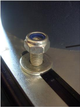
Loosen the motor mounting plate nylon locknuts and remove.
