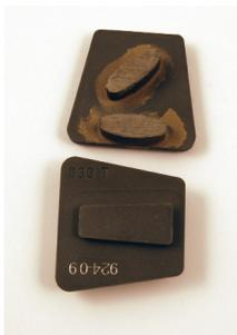
The TEQ-Lok Mini Segments provide higher contact pressure for a more aggressive grinding action. The segments are oval shaped to provide the aggressiveness of the rectangular segment with the rounded edges to minimize corner scratches in the slab surface.
