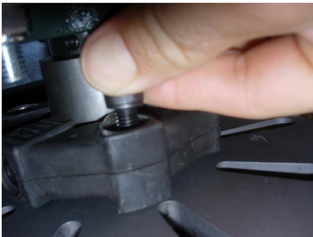
There are two common ways to change the fixed plate grinding discs, either to remove the plate from the coupler while the coupler is on the machine (see picture on Left), or to remove the coupler from the shaft from the machine and take the coupler off the disc on the bench (see picture below).
