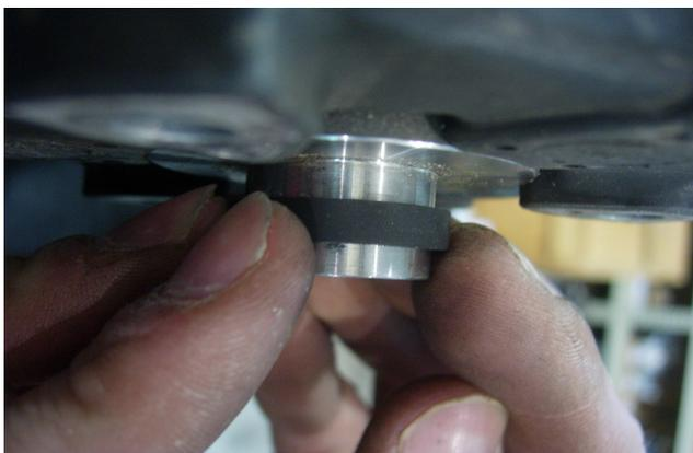
Be certain the seal is properly seated and lubricated with a Petroleum Jelly or axle grease and carefully push the disc over the shaft and seal without unseating the seal from the groove.
