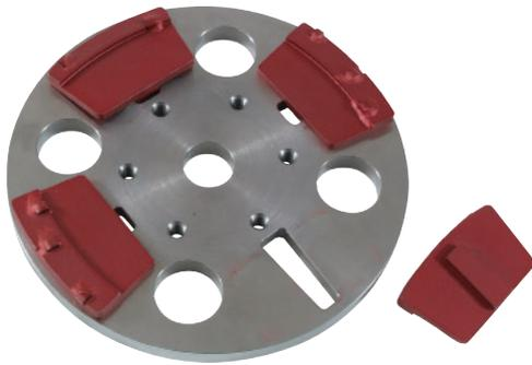
Polycrystalline diamonds (PCD's) are used for removing coatings. They are direction sensitive meaning it matters which direction they are spinning. If they turn the wrong way it will damage the PCD's. They are typically designated as Left (LH) or Right (RH) hand.
