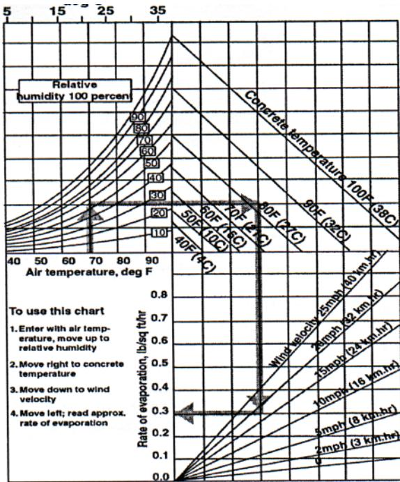
*Effect of concrete and air temperatures, relative humidity and wind velocity on the rate of evaporation of surface moisture from concrete. This chart provides a graphic method of estimating the loss of surface moisture for various weather conditions. To use the chart, follow the four steps outlined above. If the rate of evaporation approaches 0.2 lbs/sf/hr (1.0 kg/sm/hr), precautions against plastic shrinkage cracking are necessary. (lerch 1957, ACI 305).*
