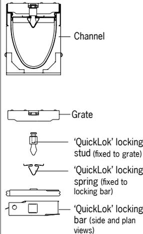
ACO 'QuickLok' is a patented boltless locking system, grates are removed and replaced with the minimum time and effort for ease of maintenance. The unique design provides a positive 'snap down' fit into the locking bar. A stud is fixed to the grate which 'locks' into the spring clip in the locking bar.
