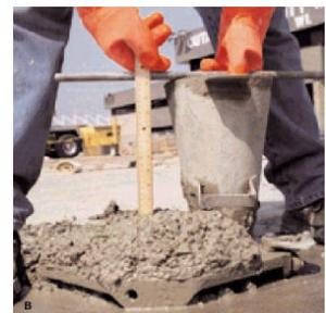
Figure 5 – Concrete mix with high slump
