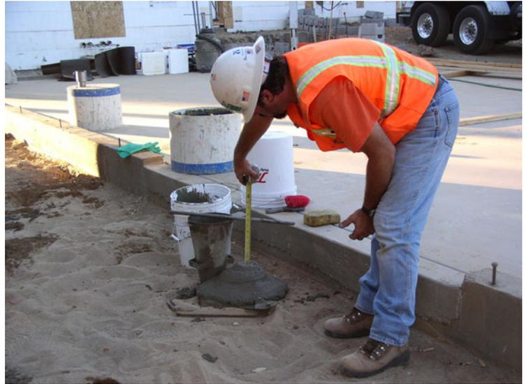
Figure 11 – Performing the slump test in the field
