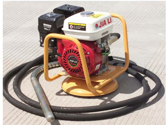
Figure 13 – Immersion type concrete vibrator with gasoline engine
