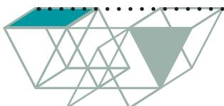
Install braces along all the wall segments at a maximum of 6' (1.8m) apart.
