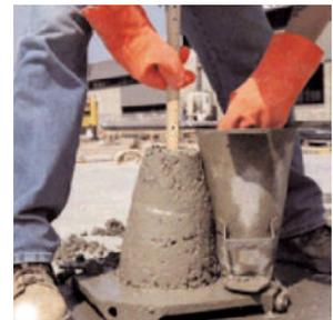
Figure 4 – Concrete mix with low slump
