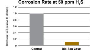
After 10 years, the concrete treated with Xypex Bio-San C500 had 9 times less corrosion than the untreated concrete, and continued to function at full efficacy.
