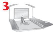
Position PointDrain on a 4" thick concrete slurry bed and ensure it is level.
