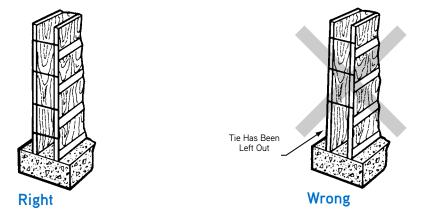
Failure to install all of the required ties or their required mating hardware will cause excessive loads to be transferred to adjacent ties and may result in form failure.
