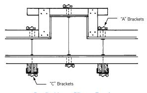
Detail of Large Pilaster Forming
