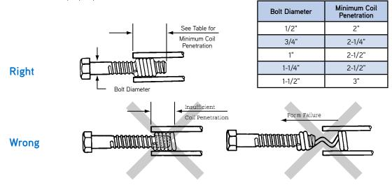
places the entire bolt load on a smaller portion of the coil welds. The increased loading can cause the coil welds to fail and result in form failure.
