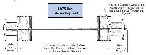
Dayton Superior A6 Spandrel Point Tie is available for tying light outside spandrel beam forms. One end is fabricated with a standard end with any style plastic cone or spreader washer. The opposite end is bent 90° with a chisel point that is driven into the deck formwork. Breakback dimension is the same as standard snap ties.
