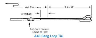
Dayton Superior A48 Gang Loop Tie is similar to the A46 tie, but has end dimensions extended to 4-15/16". The longer length allows the tie to be used with gang form bolts (supplied by others) and to be broken back before the form has been stripped. 1" breakback is standard. Other breakbacks, plastic cones and/or water resistant washers are available on special order.
