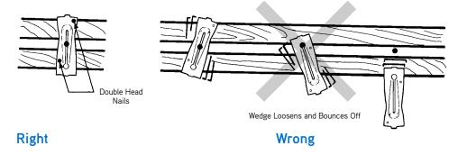
4. It is important that the snap tie head and wedge be positioned properly.
