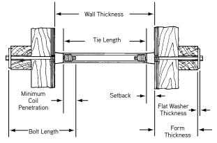
Coil Tie with Loose (Spreader) Cones
