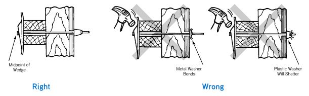
Do not attempt to draw-up warped wales with the wedge. Do not over tighten the wedge in any manner. Over tightening will cause metal spreader washers to bend out of shape or will break plastic cones resulting in incorrect wall thickness.
