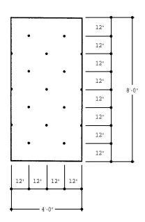
12" vertical x 12" horizontal Snap Tie spacing. Recommended rate of placement 4.5 ft./hr. at 70°.
