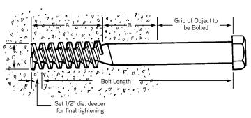
Assembled Bolt and Anchor (A&B Must Equal Ten Times Bolt Dia.)
