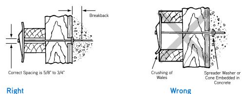
Too much space allowed between the wales may cause crushing of the wales and/or the bending of the wedge allowing the form to bulge outward. This results in incorrect wall thickness and causes the tie spreader washers or cones to become embedded and trapped in the concrete. Trapped tie washers or cones will cause difficulties during the tie breakback operation.
