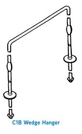
single or double ledgers. This secures the beam bottom against the spreader washers to provide a rigid form and correct depth of fire-proofing. C1C Wedge Hangers (without spreader washers) are recommended for use only with soffit spacers.
