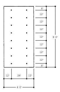
12" vertical x 24" horizontal Snap Tie Spacing. Recommended rate of placement 4.5 ft./hr. at 70°.
