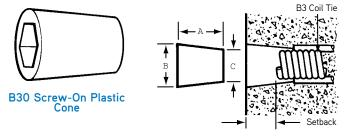
Warning: Cones are to be used for spreader action only and are not designed for scaffold bracket or other accessory loads.
