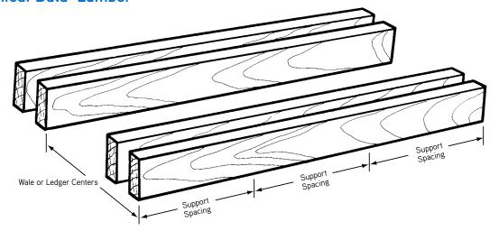
Safe Spacing of Supports for Double Ledgers or Wales Continuous Over Four or More Supports
