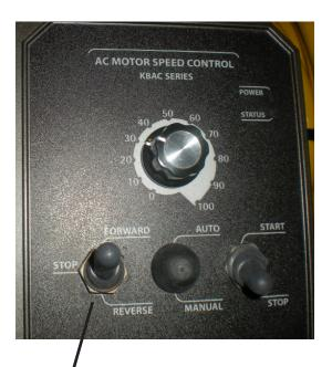
On variable Speed models, be certain the proper rotation for the PCD is made via the FWD/REV switch.
