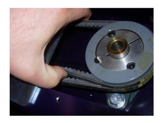
The proper tension of the belts are established by the belt manufacturer. A rule of thumb is that if you can squeeze the belts as shown with a deflection about the thickness of the belt, it is probably close to the proper tension.
