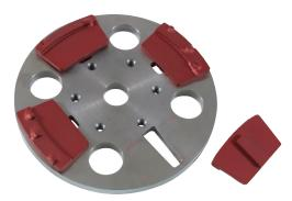
Polycrystalline diamonds (PCD's) are used for removing coatings. They are direction sensitive meaning it matters which direction they are spinning. If they turn the wrong way it will damage the PCD's. They are typically designated as Left (LH) or Right (RH) hand.
