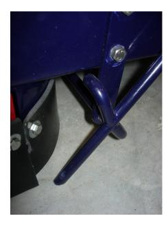
The Gasoline Powered models have a kickstand option to lift the grinding head off the ground so the engine can be started without the extra load of the disc resisting.
