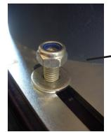
Loosen the motor mounting plate nylon locknuts and remove.
