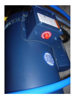
The thermal overload on the motor is located under the motor conduit box (see picture to the left for Leeson and below for Baldor). Be certain the thermal overload and motor are fully cooled before reseting the overload.
