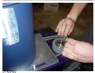
Tighten the belt tensioning bolt until the belts are properly tensioned.
