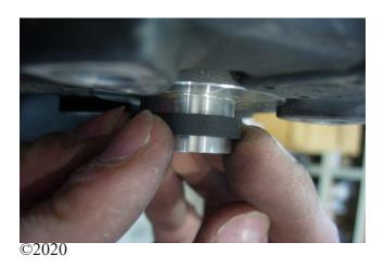
Be certain the seal is properly seated and lubricated with a Petroleum Jelly or axle grease and carefully push the disc over the shaft and seal without unseating the seal from the groove.
